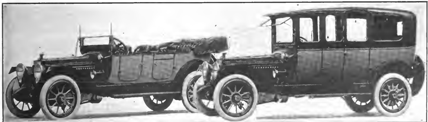
Fig. 6—Left—Packard 3-38 touring chassis with six passenger saloon touring body. Right—Touring chassis with limousine body
